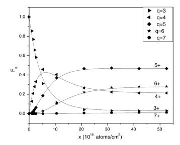
Fig. 3. Charge-state fractions as a function of target thickness for an 9.6 MeV  $O^{3+}$  beam in He. The solid lines are CSDsim predictions using the fitted cross-sections (see text). The data shown are results from [6].
