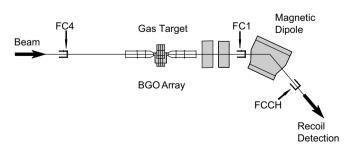
Fig. 1. Diagram of the relevant components of the DRAGON apparatus for the beam CSD measurements. FC denotes a Faraday cup.
